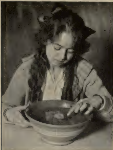
FIG. 106. A compass made of a needle and a piece of cardboard.
